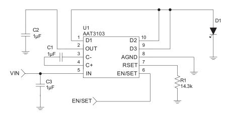
Figure 6: Higher Current, Single LED Application.
