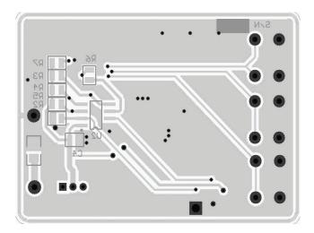
Figure 10: AAT3103 Evaluation Board Bottom Side PCB Layout.
