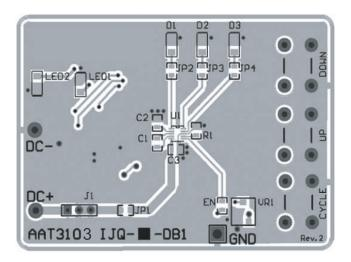
Figure 9: AAT3103 Evaluation Board Top Side PCB Layout.
