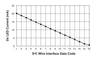
Figure 2: AAT3103-1 Current Control Profile,  $R_{SET} = 14.3k\Omega$ .
