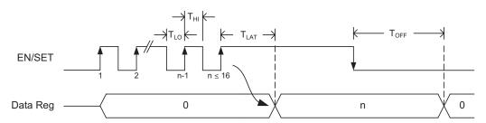
Figure 1: S<sup>2</sup>Cwire Serial Interface Timing.
