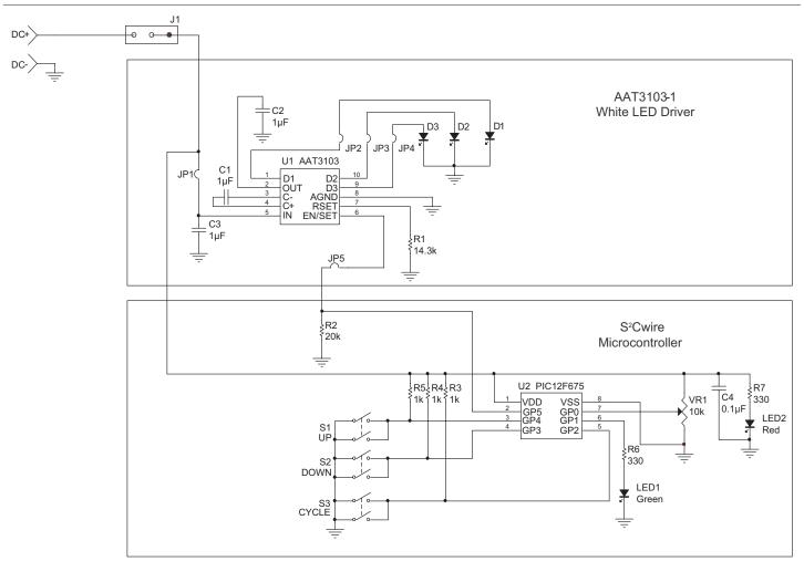
Figure 8: AAT3103 Evaluation Board Schematic.
