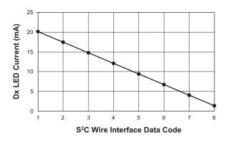
Figure 3: AAT3103-2 Current Control Profile,  $R_{\text{SET}} = 14.3 \text{k}\Omega$ .
