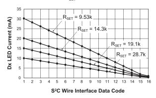
Figure 5: AAT3103-1 LED Current Control Profile at Different  $R_{\text{SET}}$  Values.
